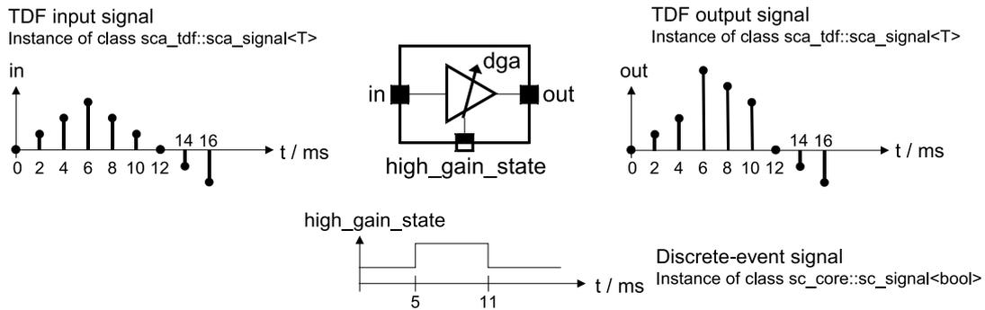
Figure 2.26. TDF module with a converter port used as control input
