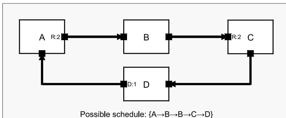
Figure 2.6. Multirate TDF model with loop
