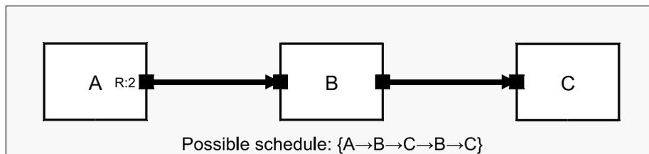
Figure 2.3. Multirate TDF model using port rate assignment
