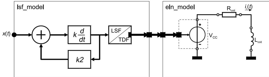
Figure 7.7. Coupling of LSF and ELN via an LSF/TDF converter module
