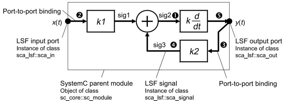
Figure 3.3. Port binding rules for LSF input and output ports
