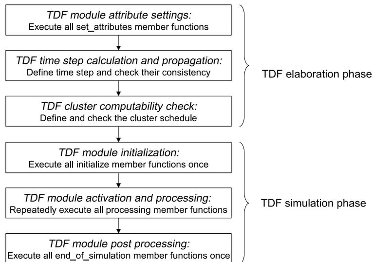
Figure 2.27. TDF elaboration and simulation phases
