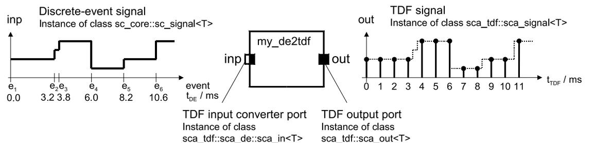
Figure 2.24. TDF module with converter port as input
