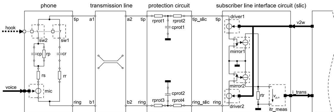
Figure 4.11. The Plain Old Telephone System (POTS) front-end
