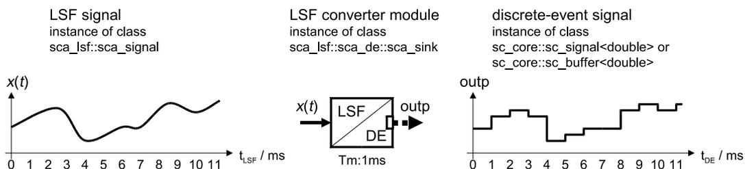
Figure 3.6. LSF converter module reading from an LSF input signal and writing to a discrete-event output signal
