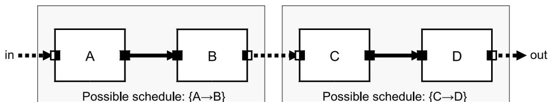
Figure 2.14. Use of TDF converter ports to deliberately split a cluster in two independent ones
