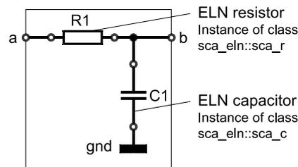
Figure 4.4. ELN circuit implementation of a first-order low-pass filter
