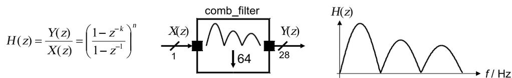
Figure 5.3. Frequency response of a comb-filter implemented in the z-domain
