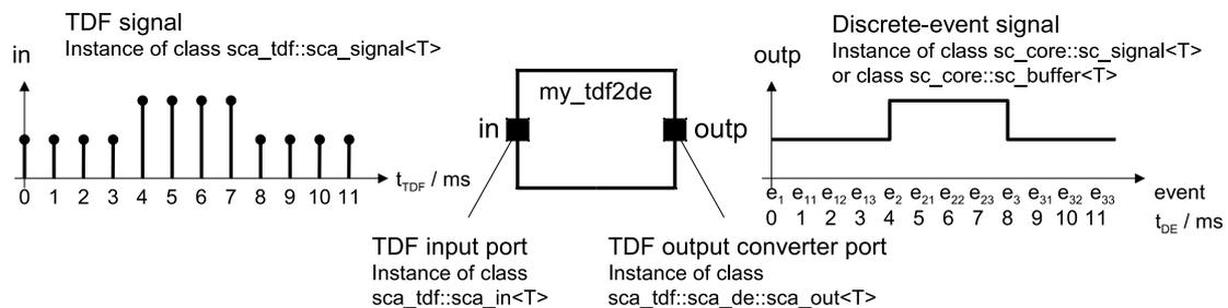
Figure 2.25. TDF module with a converter port as output
