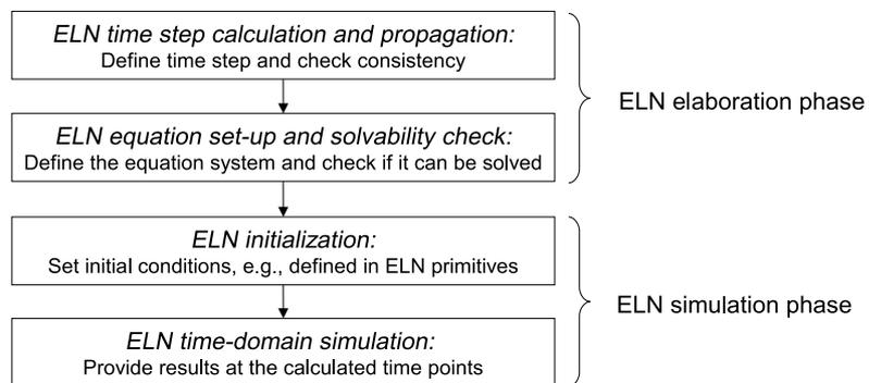
Figure 4.10. ELN elaboration and simulation phases
