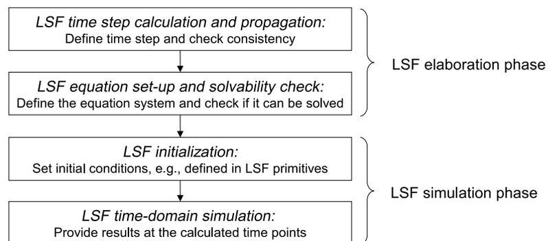
Figure 3.11. LSF elaboration and simulation phases
