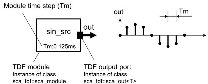
Figure 2.16. TDF primitive module implementing a sinusoidal source
