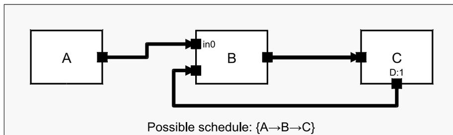
Figure 2.5. TDF model with loop, and port delay assignment
