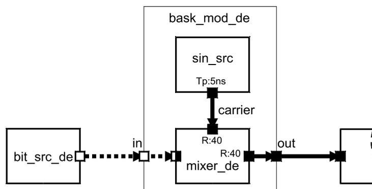
Figure 2.30. BASK modulator, mixing discrete-event and TDF domain
