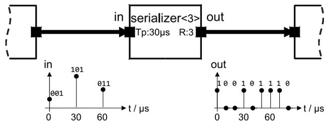
Figure 7.11. Serialization of a 3-bit vector
