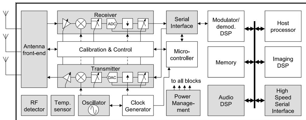
Figure 1.1. A Communication System, example of an embedded analog/mixed-signal architecture
