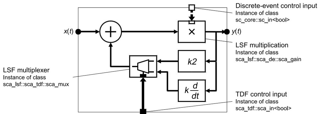
Figure 3.9. LSF model using discrete-event and TDF control signals
