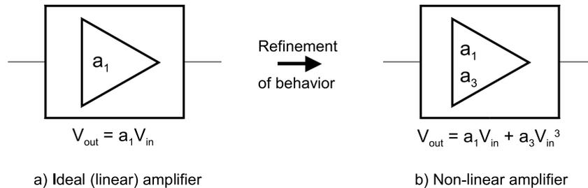
Figure 7.9. Refinement of behavior of an amplifier
