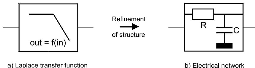
Figure 7.10. Structural refinement of a filter
