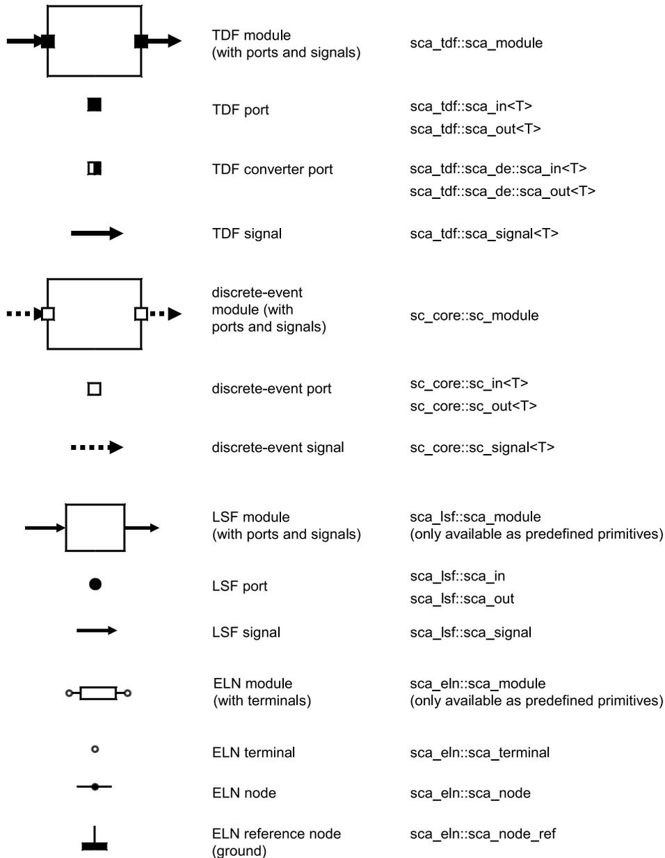
Figure B.1. Symbols and graphical representations of TDF, LSF, ELN and discrete-event elements.
