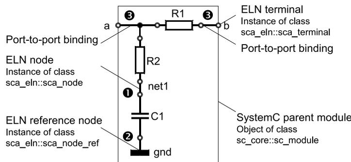
Figure 4.3. Port binding rules for ELN terminals
