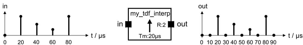
Figure 2.21. Multirate example: 2 times oversampling by inserting zeros
