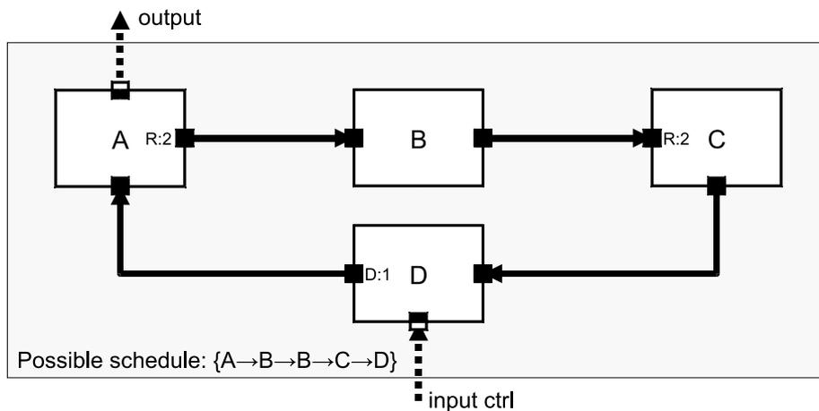
Figure 2.8. TDF model interfacing with discrete-event domain
