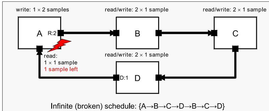
Figure 2.7. Multirate TDF model containing a loop with incompatible rates, resulting in accumulation of samples in the cluster yielding to an infinite (broken) schedule
