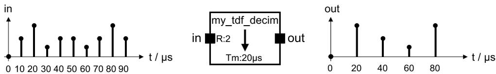
Figure 2.22. Multirate example: Downsampling by a factor of 2
