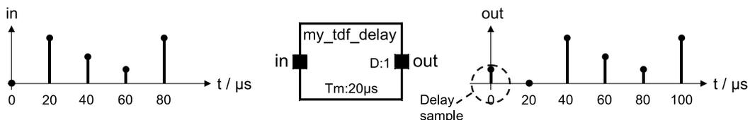
Figure 2.23. TDF module introducing a delay of one sample
