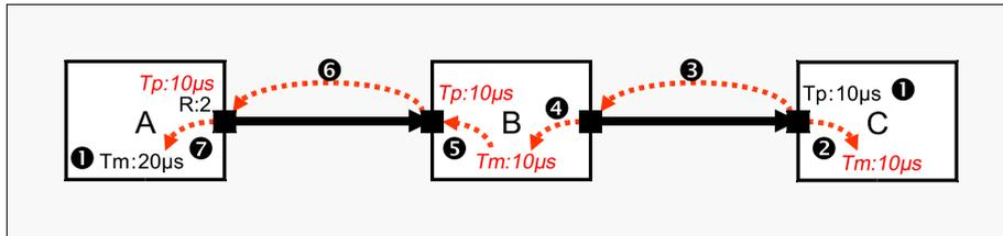
Figure 2.12. Time step propagation for a multirate TDF model with consistent time step assignments done by the user
