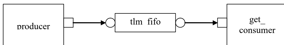
Figure 6—Using a uvm_tlm_fifo
