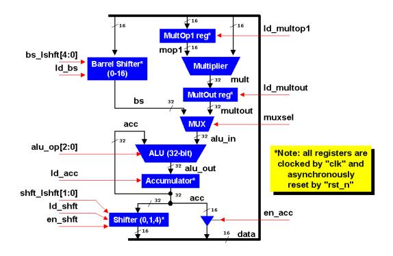
Figure XXX - Block Diagram of a Complex Arithmetic Logic Unit (CALU) (A black & white version of this gif diagram will be provided if we pass this enhancement and decide to keep this example)
